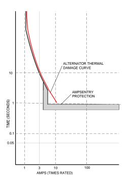
**Short circuit shutdown** - Output current on any phase is more than 110%, more than 175% of rating, and approaching thermal damage point of alternator. Control includes algorithms to protect alternator from repeated over current conditions over a short period of time.
