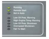
The operator panel includes a series of LED indicating lamps to allow the operator to view the general status of the generator set. Functions displayed include:
