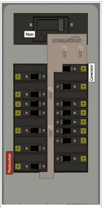
This Interlock Kit mounts to SQUARE D electrical panels with the following features:
